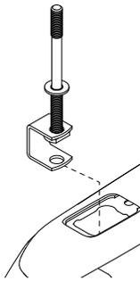
Remove rear stake pocket cover, install rear stake pocket bolt by hooking under bracket inside pocket. Hand tighten the stud thru the hole until the washer (welded to the stud) bottoms out.
