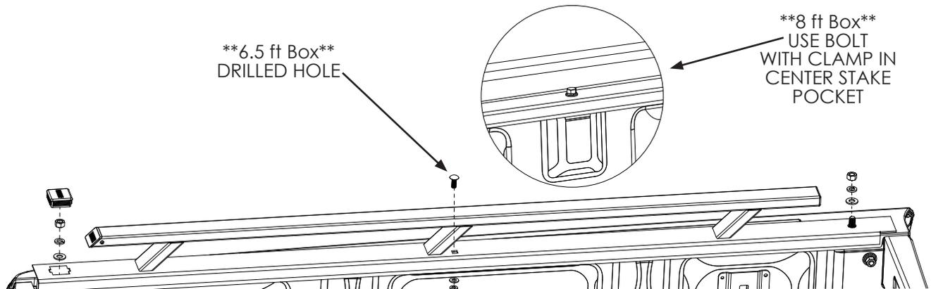
Place side rail over the stake pocket bolts (5.5 and 6.5ft) . Hand tighten all bolts. Align side rail against inside and front of truck bed. Torque all bolts. Snap trim cap into rear square hole.
